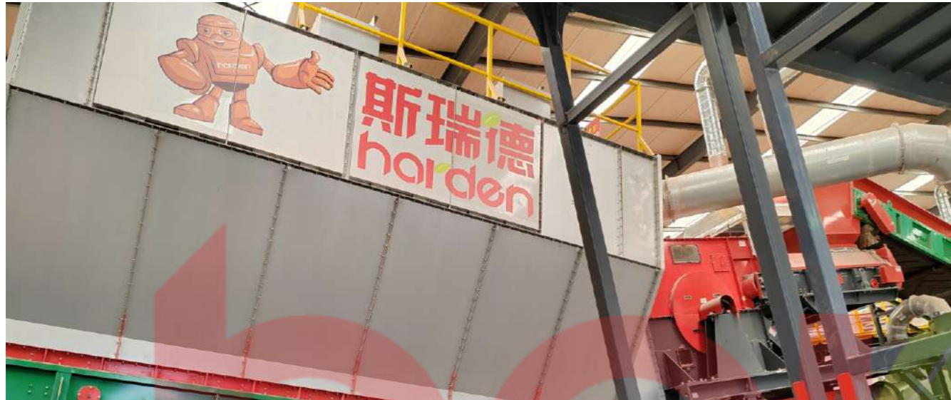
Processing materials: Industrial Waste Site: Taiwan Date: July 2023 Model: SFX800 (8t/h, 80-200mm) Application: Removing impurities from RDF fuel
